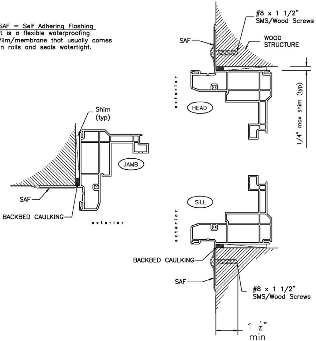
**Figure 9: Installation type "D" using Fin Frame**
