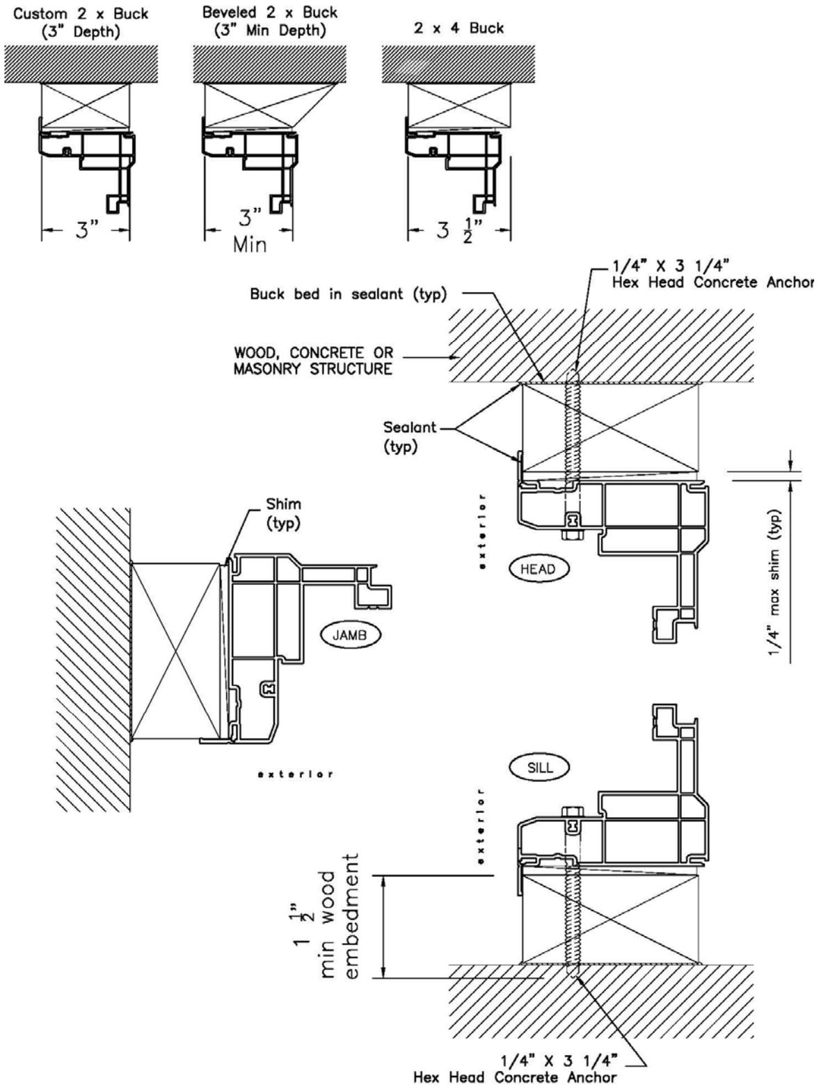
**Figure 5: Installation type "B" using 2 x bucks**
