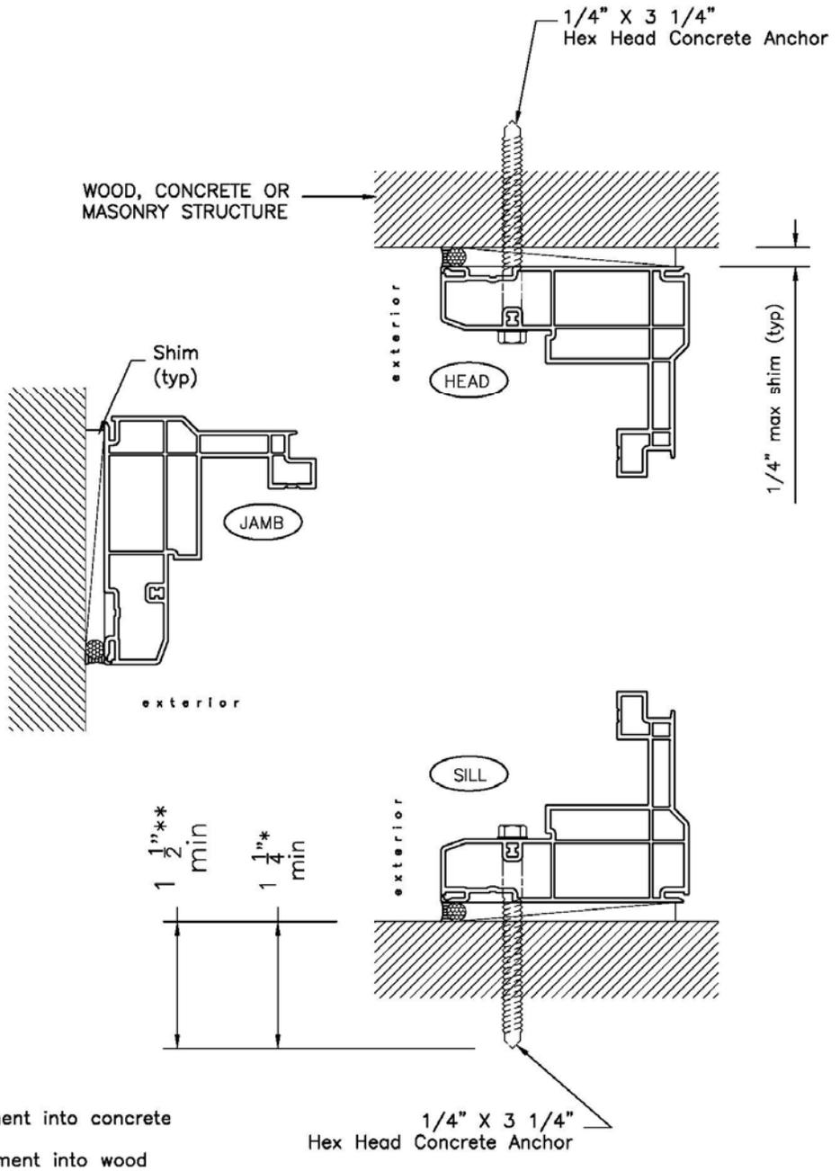
**Figure 6: Installation type "C" using 2 x bucks using Equal Leg (Flush) Frame directly into structure**
