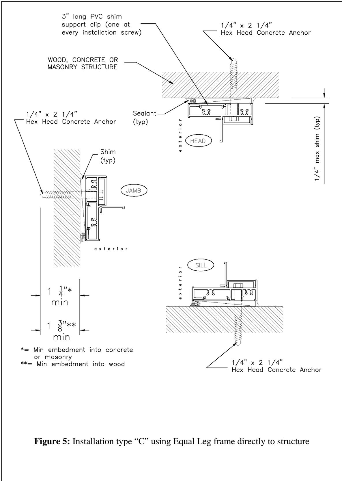
**Figure 5:** Installation type "C" using Equal Leg frame directly to structure
