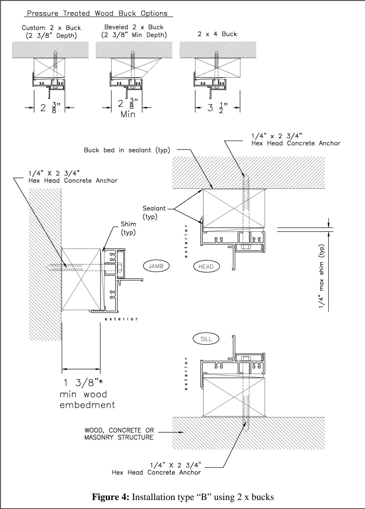
**Figure 4:** Installation type "B" using 2 x bucks
