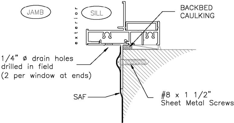
Figure 6: Installation type "D" using Fin Frame
