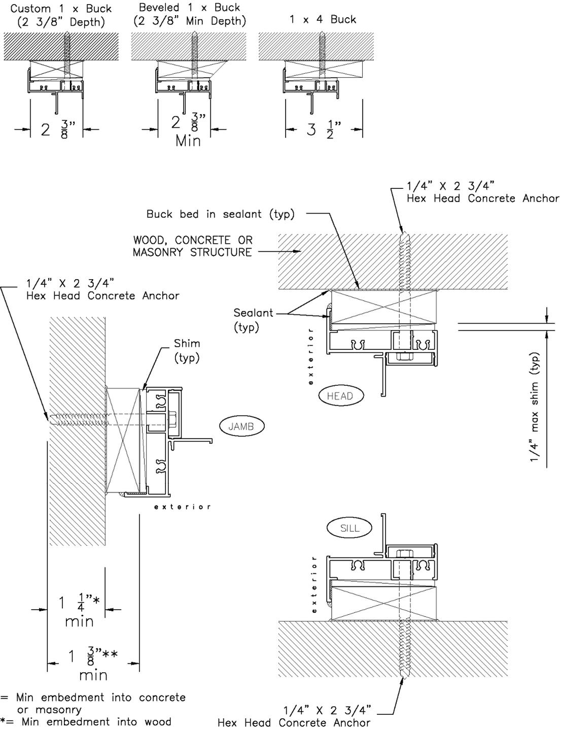
**Figure 3: Installation type "A" using 1 x bucks**
