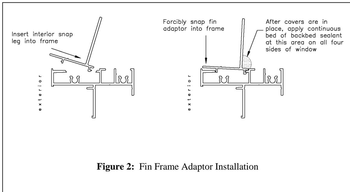
6. Stand window upright. Add a generous amount of backbed sealant (minimum 3/8” bead) to the backside of the fin adaptor as shown in figure 2. This seal is **CRITICAL**, especially at the sill area. This seals between the adaptor & the frame and between the window & the opening. Add this sealant to the head, sill and jambs. Install window from the outside into wood opening.
